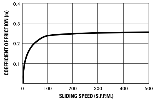
COEFFICIENT OF FRICTION VS. SPEED (AT 100 P.S.I.)
